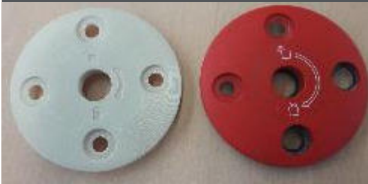
Door Lock printed in ASA
