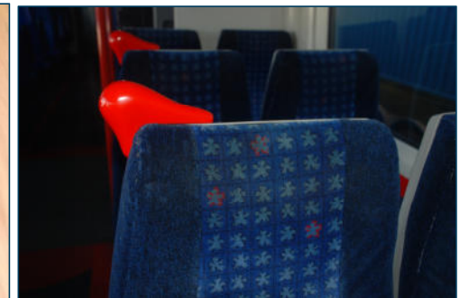
Red Grad handle 3D printed in ULTEM™ 9085 resin after 3 months trial
