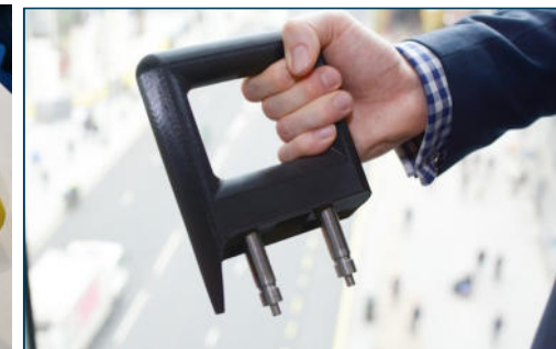
Red Grad handle 3D printed in ULTEM™ 9085 resin after 3 months trial
