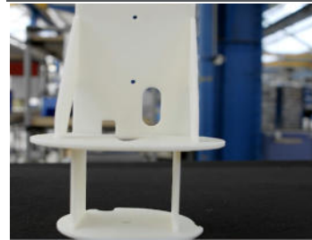
Lamp Holder in ABS instead of sheet metal
