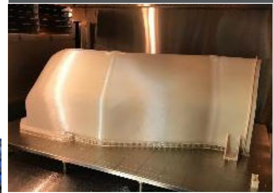
External Duct in ULTEM™ 9085 resin
